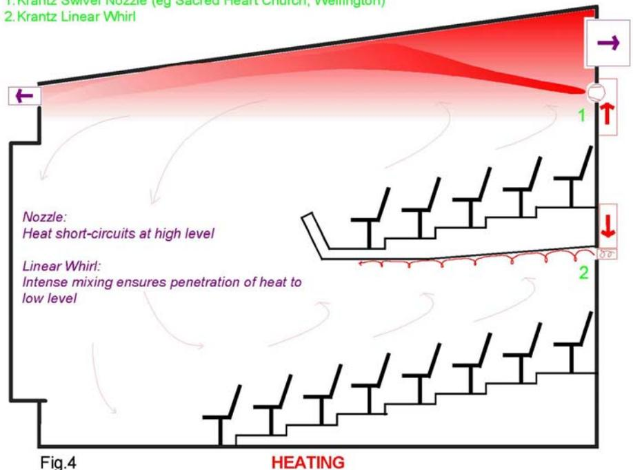
Rather than blowing unsteady masses of air into open spaces, or sucking such unstable bundles to ceilings by means of Coanda-effect attachment, high velocity nozzles can be used to concentrate supply air into narrow jets that are shot across high level open spaces. The high momentum of each jet stabilises and extends the cold or warm supply streams' otherwise limp trajectories, eliminating icy dumping onto unsuspecting occupants or plumes of supplied heat from ineffectively wafting
